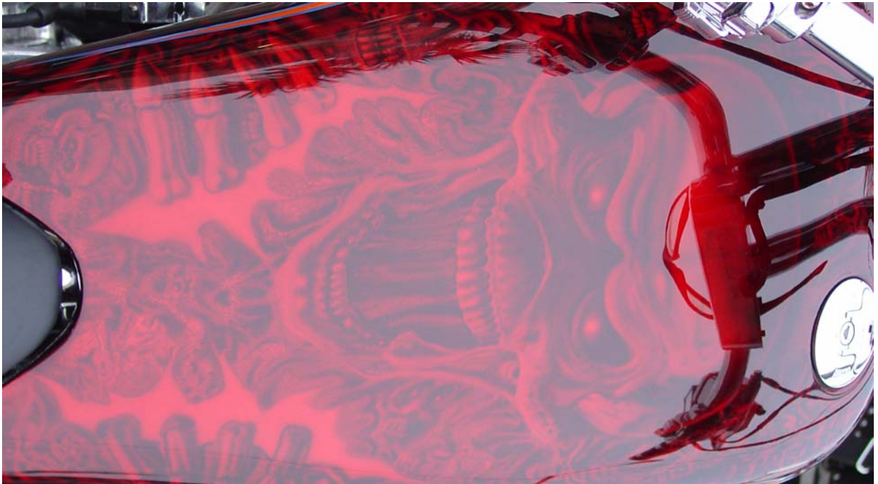
FIG 1: This graphics job was painted using an Iwata airbrush and black basecoat, then covered with 3 heavy layers of urethane candy red. When using candy to paint graphics, it is recommended to use “intesifier” candies mixed into a clear basecoat. This will keep the colors thin and clean. This job was completed over a weekend.
